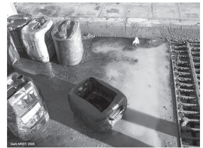
At a garage in Hebron, makeshift oil pans are used to drain car oil, which is disposed through the grille into the sewer. All Hebron sewage flows untreated into the Hebron River.
